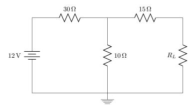
To measure the Thevenin Resistance we need to remove the power supply and replace it with a wire. The load is produced by measuring the resistance with your multimeter.
