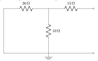
$$R_{TH} = (R_1 || R_2) + R_3 = 30\Omega || 10\Omega + 15\Omega = 7.5\Omega + 15\Omega = 22.5\Omega$$
