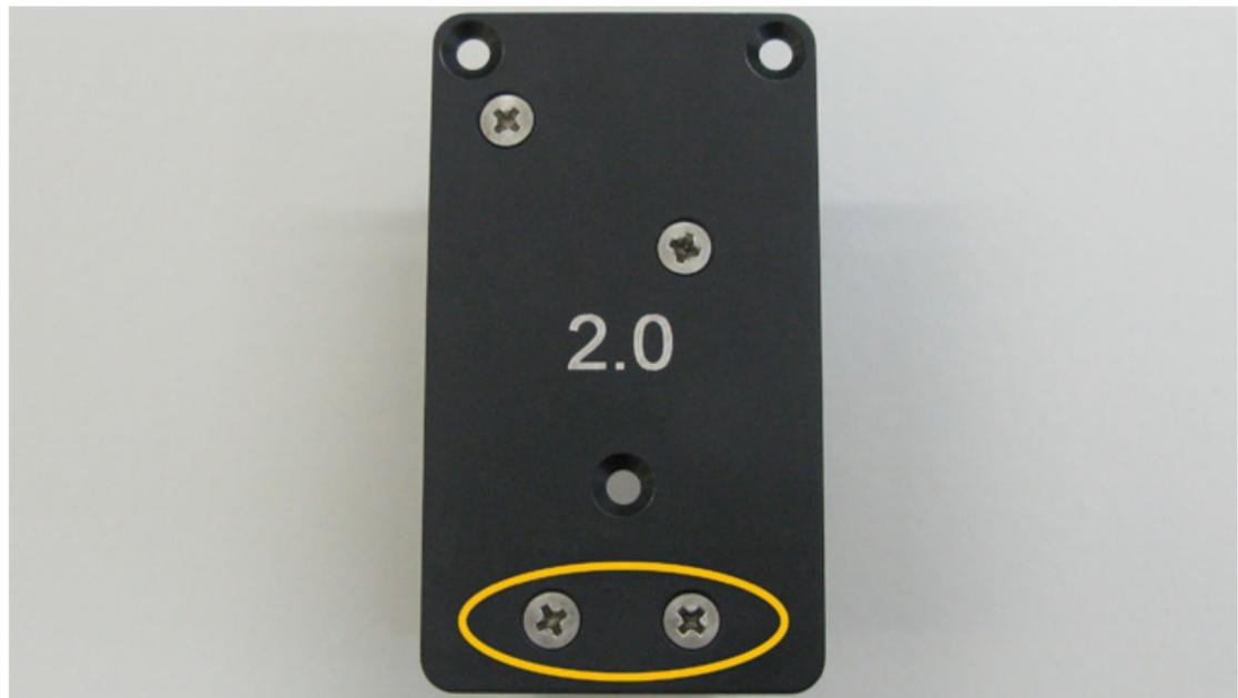
8. Attach the new Focusing Lens to the Front Cover Plate. Leave the Phillips head screws slightly loose.
