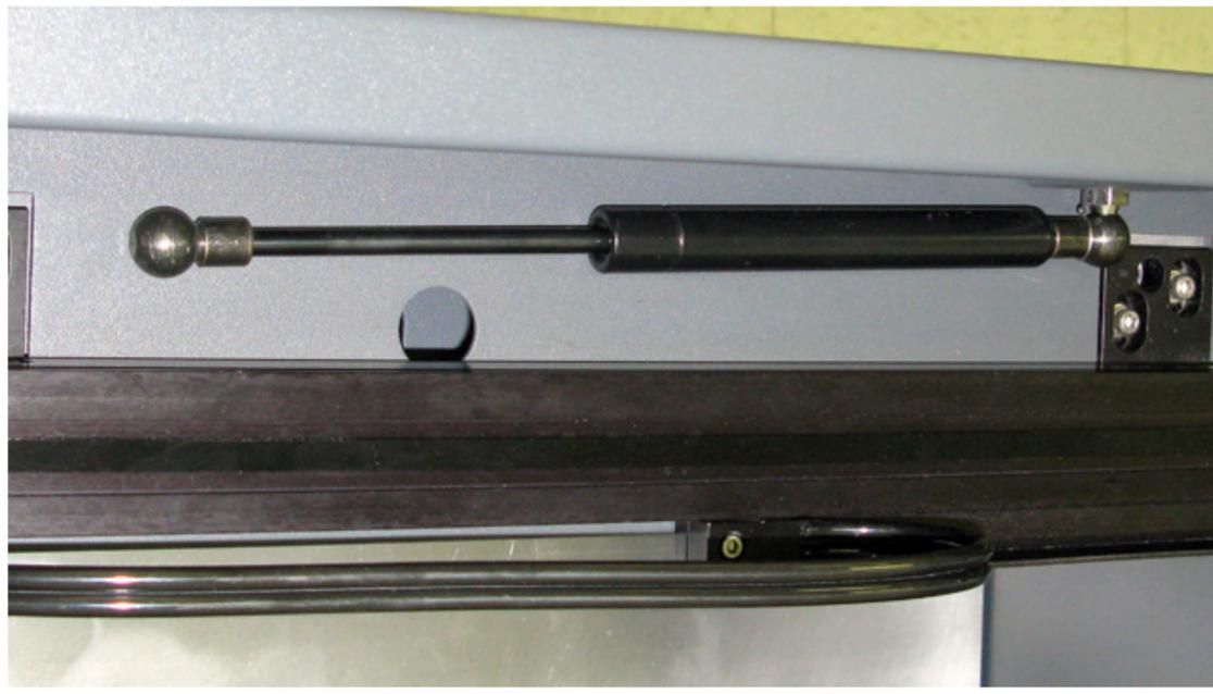
5. With another person holding the top door remove the four screws and washers that hold the top door in place. Set the top door in a safe location and set the screws and washers safely aside.
