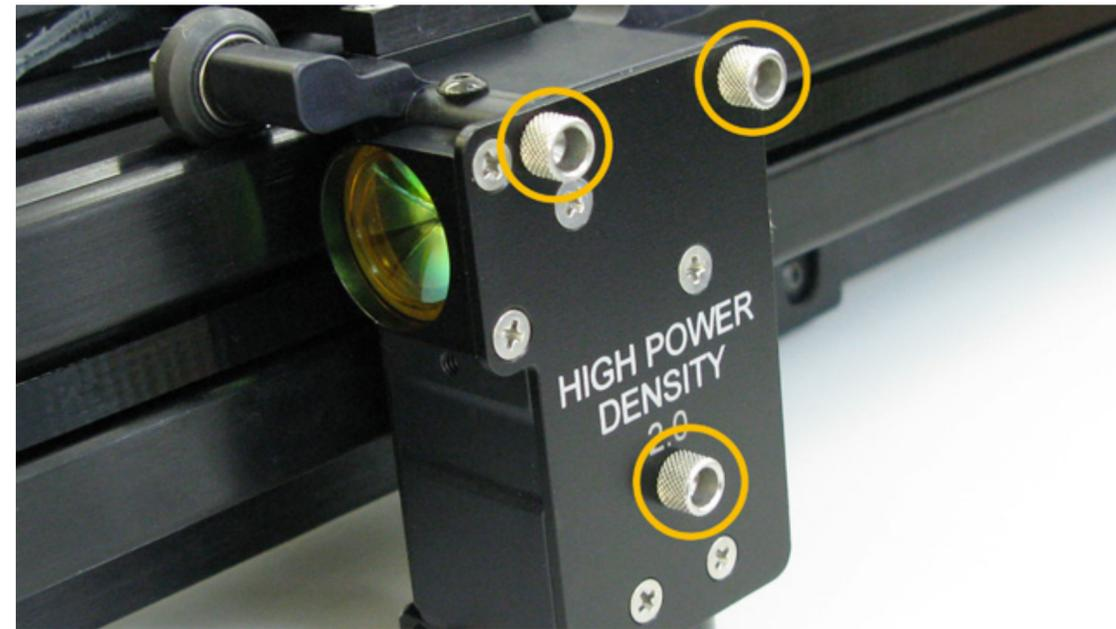
5. Slide the Lens Kit out of the Focus Carriage.
