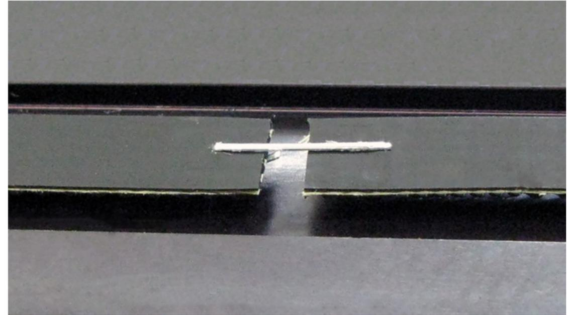
6. Pull the other end of the old belt, allowing the new belt to be pulled through the inside of the Y-axis Rail. Make sure you do not twist the belt as it goes through the rail. The teeth of the belt should face inward.
