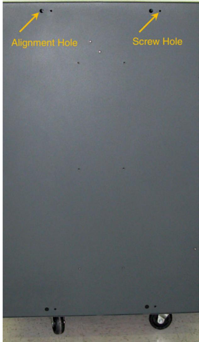
4. Using the two remaining screws, flat washers, and locking washers, attach the back panel to the rear of the system.
