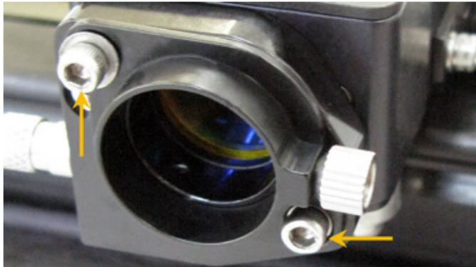
9. Tighten the base mounting screws gently and re-check the cone's alignment.
