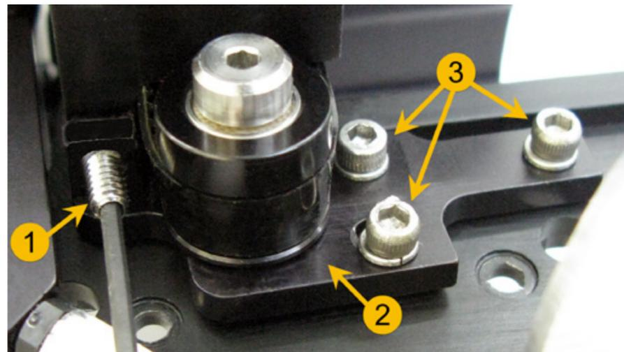
5. Once the tension has been released remove the screw on the Idler Pulley. Remove the pulley, paying attention to the orientation of it, and replace it with a new one.
