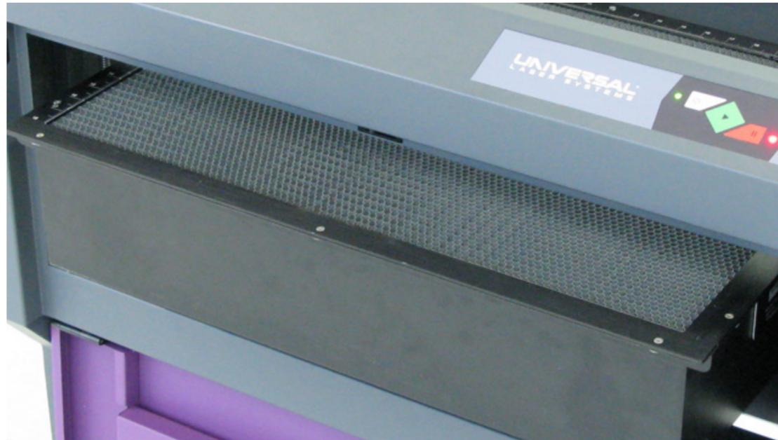
3. The rulers of the cutting table should overlap the rulers on the engraving table.
