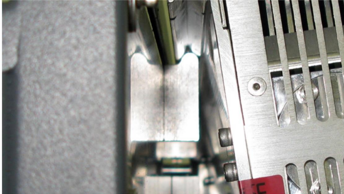
8. When rotating the laser down, make sure there are no obstructions, such as cables that could be pinched. At the end of the rotation you should feel a slight click and the laser should be completely parallel to the back plate of the system.
