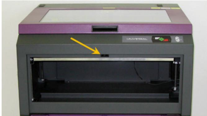
2. Locate the front door latch catch(es) noting the direction the imprinted arrows are pointing.
