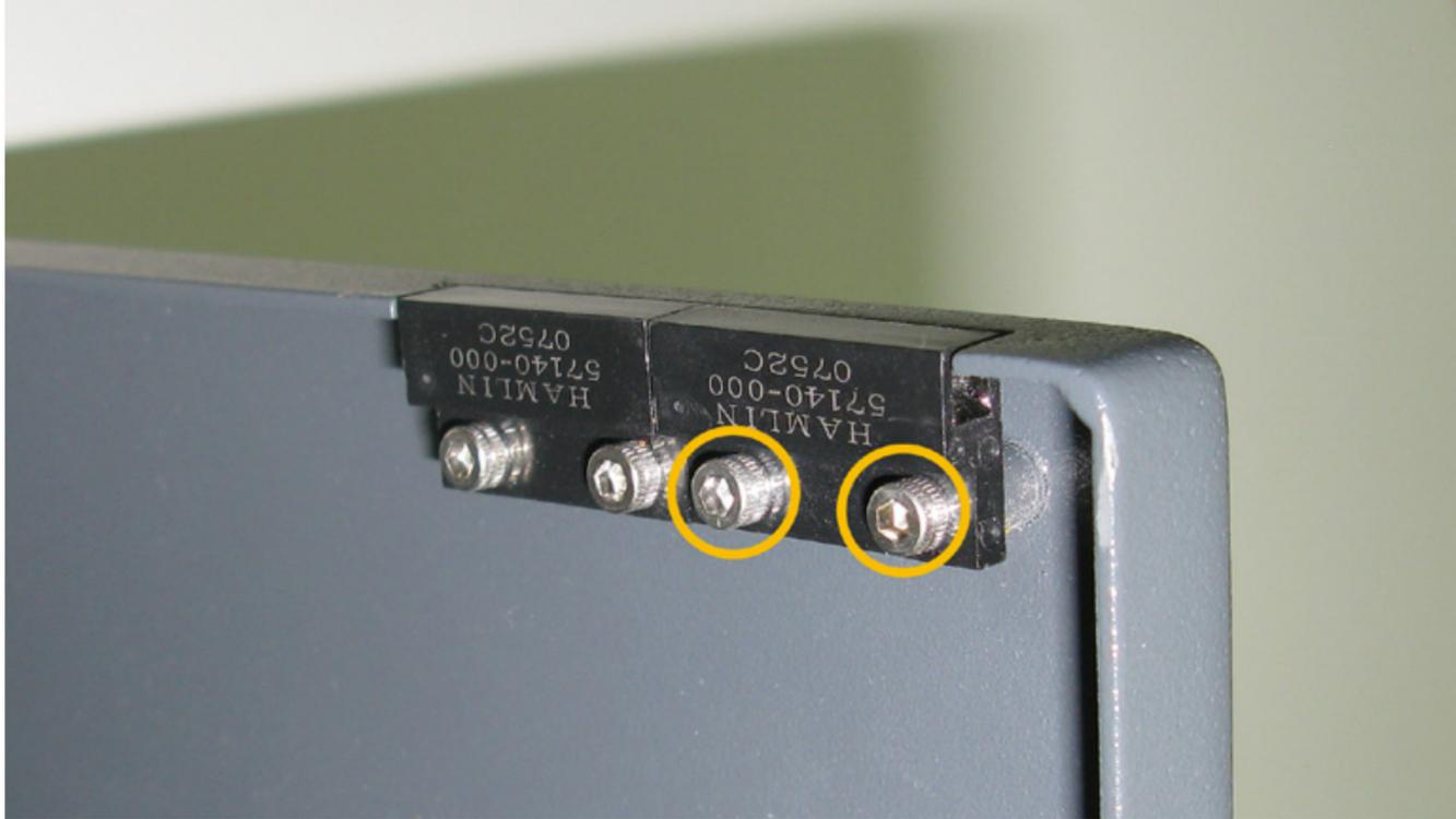
6. Installation is opposite of removal. Ensure that the proximity sensor magnet is flush with the rear cover.
