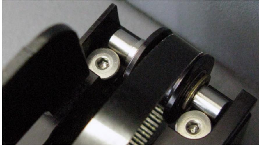
4. On both Y-axis Rails is a Y-axis Belt Clamp. Unscrew all 6 screws, 3 on each, and set the screws and clamp aside.
