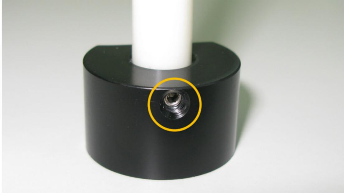
14. Raise and/or lower the shaft of the focus tool until the distance between the base of the tool and the notch is in perfect focus with the carriage as it was set in step 12.
