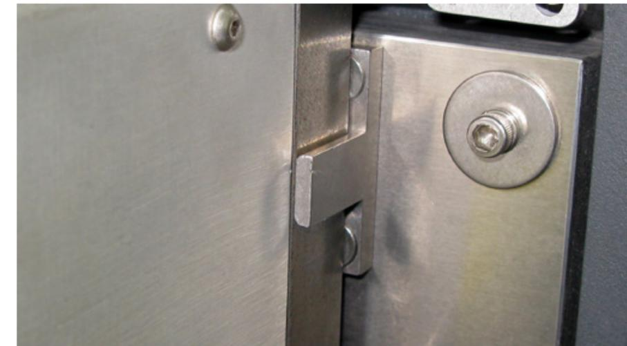
7. With the laser at an angle make sure it is hanging correctly on the two laser supports while still seated on the alignment fork correctly.
