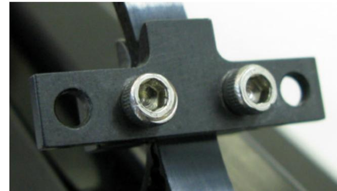
6. Remove the right end support by removing the four screws located on the top (2) and bottom (2) of the support.
