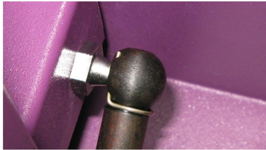
3. Once the retaining clips have been removed the hydraulic pressure cylinders can be removed by pulling outward from the door/system.
