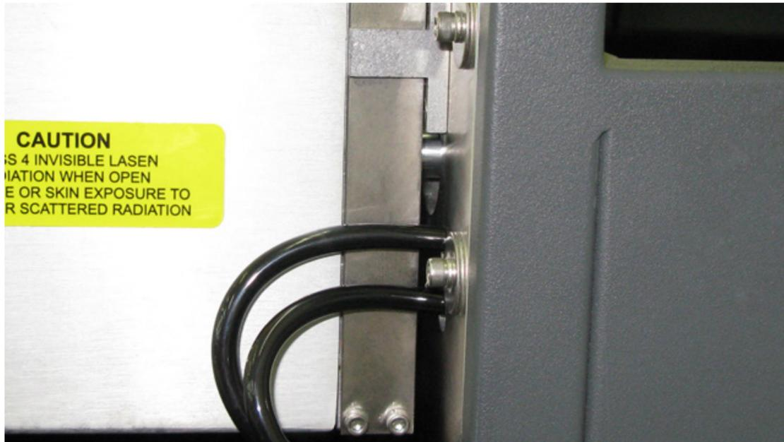
9. Plug the electrical connector to the back of the laser as removed in step 3.
