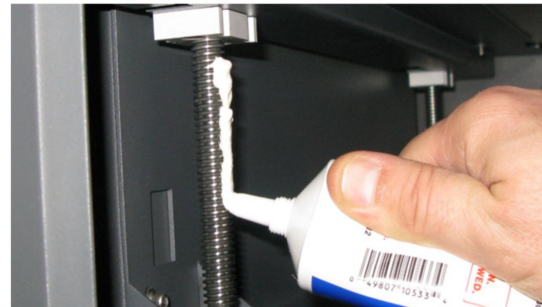
19. Plug in and turn the system ON. Run the Table up and down to work in the grease. Once the table is running smoothly, re-home the Z-axis.
