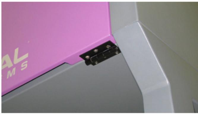
7. Plug in and power ON the VLS. Open and close the door. Check to see if the door open light on the keypad turns on and off (red flashing light) when you open and close the door. Or check the UCP to see if the system is indicating that a door is open.
