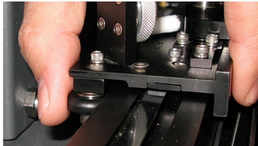
**NOTE:** You should feel an equal turning resistance for each bearing. If one bearing spins freely and the other has a turning resistance, or the turning resistance is unequal, then adjustment is necessary.
