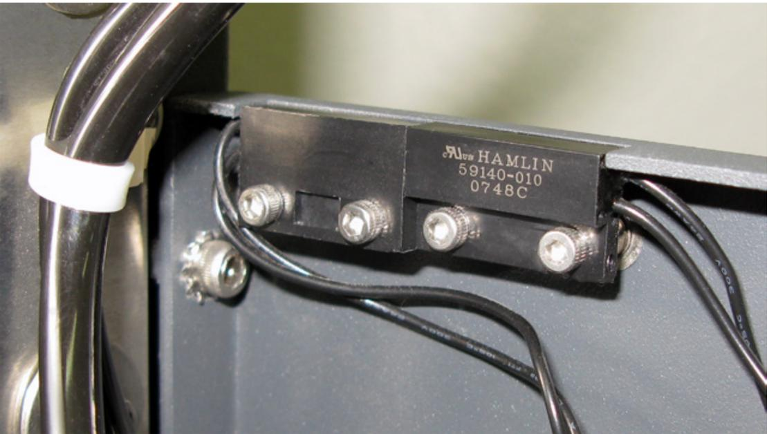
4. Disconnect the interlocks from the wiring harness.
