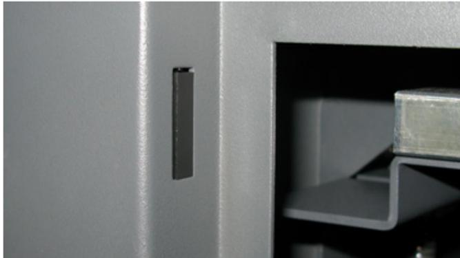
5. Disconnect the proximity sensor from the wiring harness.
