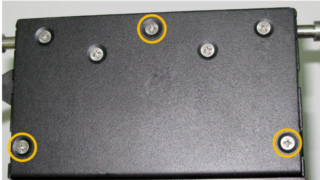
3. Turn the rotary back over and remove the cover by pulling straight up.
