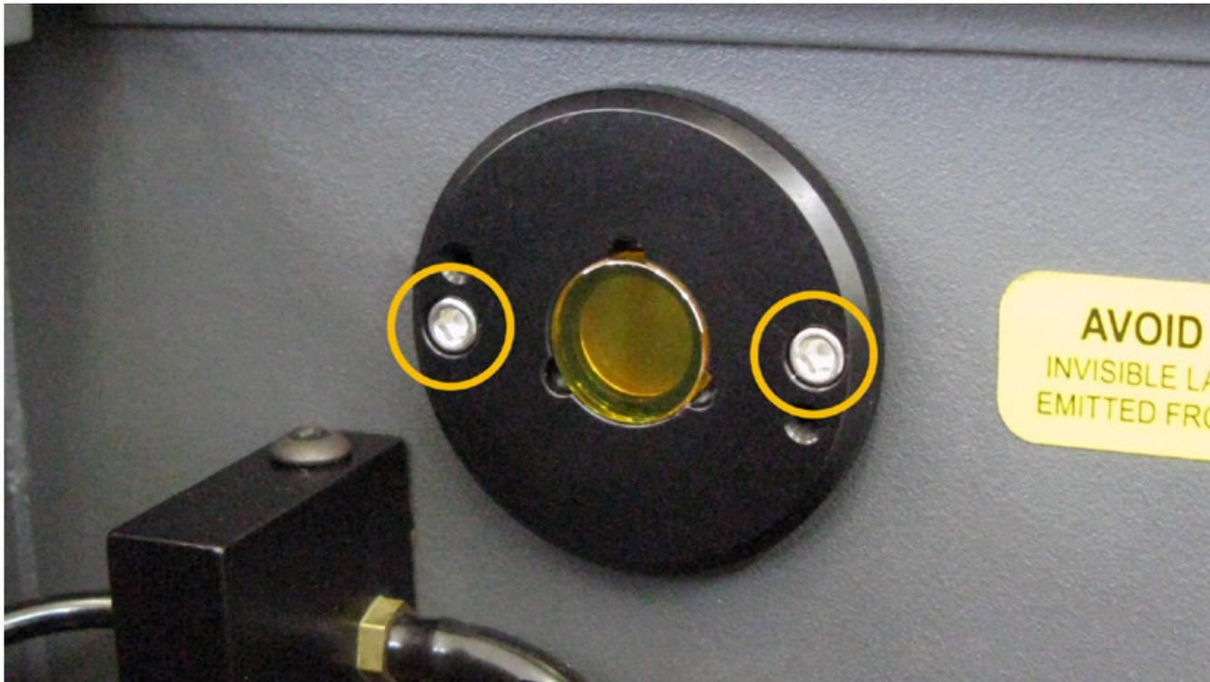
4. Carefully remove the Beam Window.
