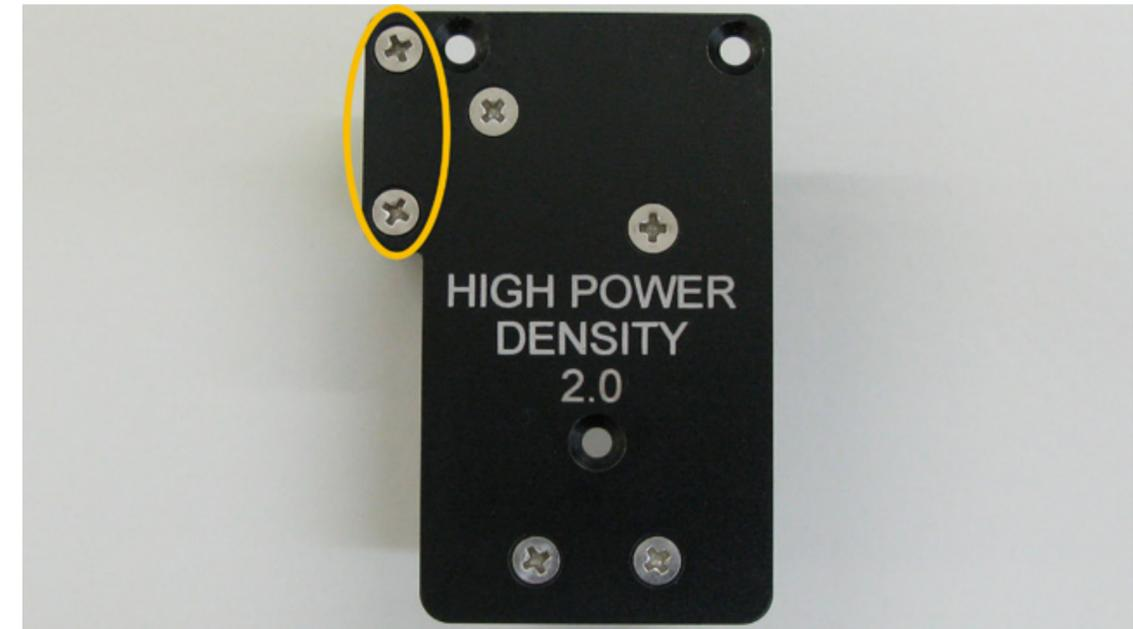
8. Attach the new Beam Shaper to the Front Cover Plate.
