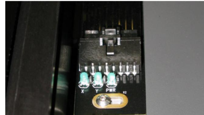
5. Unscrew the 2 screws that hold the board and set side in a safe place.
