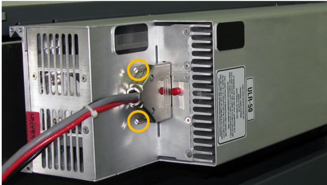
4. Rotate the laser a few degrees to the outside from the bottom and lift it up and off the mounts. Store the Laser in a safe place.
