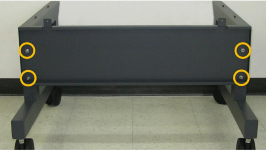
3. With the assistance of another person, place the system on top of the cart, aligning the pins on the cart with the alignment holes on the bottom of the system, and loosely install the 4 socket head screws, 4 locking washers, and 4 flat washers attaching the system to the cart. These screws will go through the cart legs into the bottom of the system.
