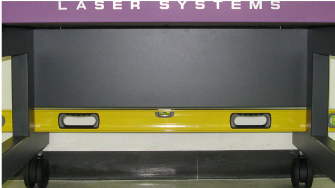
9. Once the system is level tighten the appropriate locknuts.
