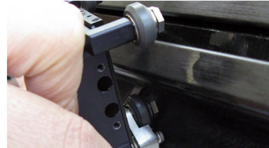
7. Hold the Focus Carriage or place it on a flat surface facing down and remove all 3 bearings.
