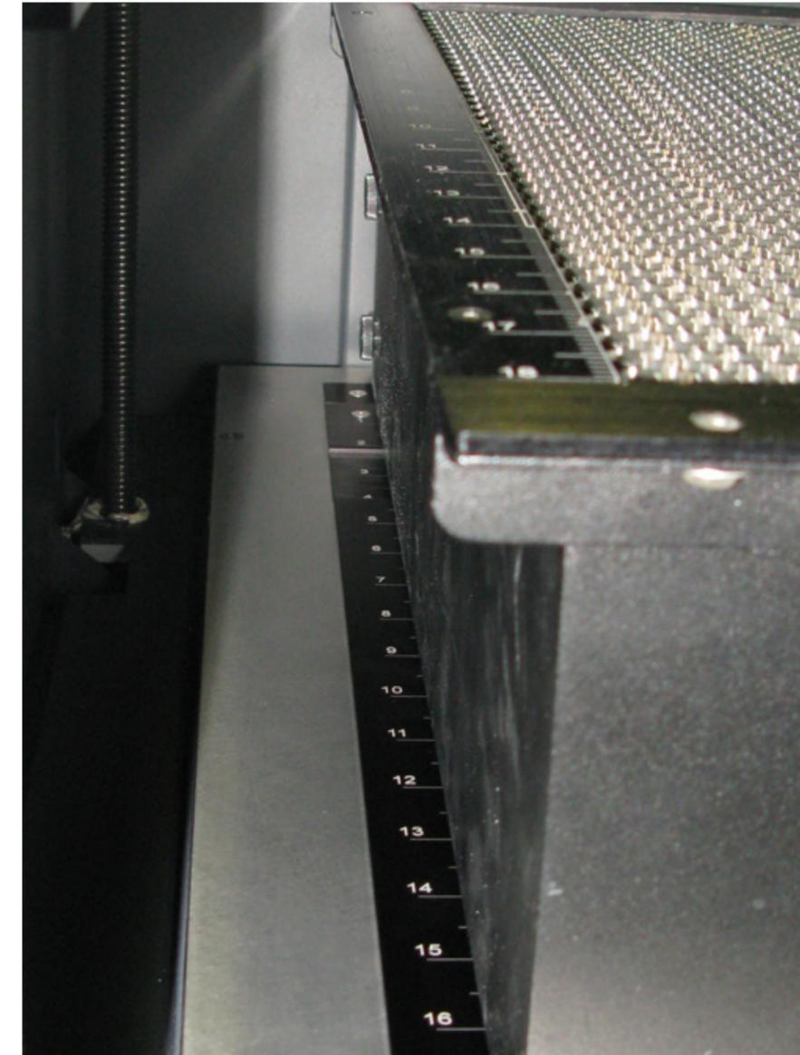
**NOTE:** The front left foot of the Cutting Table is offset. If you try to press both the front and rear left feet against the Y-Axis ruler, the Cutting Table will not be square to the engraving table.
