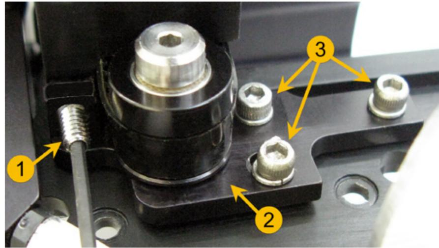
4. On the right end of the arm remove the two screws and the two washers that attach the motor bracket to the X-axis rail. Remove the motor assembly from the arm.
